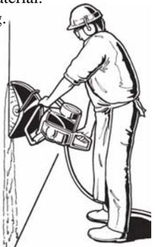
**Cutting blades:** Always use the type of blade that will cut the material with the least amount of effort. Standard abrasive blades can be used to cut softer material such as aluminum. Carbide blades can be used to cut mild steel, or diamond impregnated blades can be used to cut very hard material such as concrete or titanium.
