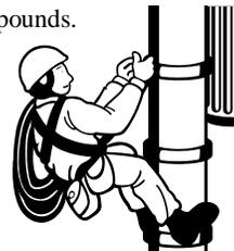
**Conclusion:** Personal fall arrest systems and positioning devices systems components must be inspected prior to each use, and after any fall or incident for damage, wear, deterioration, or defective components.
